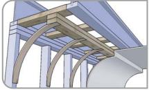
Top Reveal- At each corner of the room measure and mark the wall down from the ceiling <u>14</u> inches plus the thickness of your reveal (rise). Measure and mark the ceiling out from the wall <u>14</u> inches (rise).
