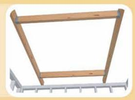
Using a tape measure and square, measure and mark center lines on all four sides of your 5'-0" square box (2'-6" or 30" in from each corner).
