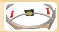
Nail or screw the miter ends of the 2 dome rafters into the dome ring using 2 nails or screws per dome rafter.
