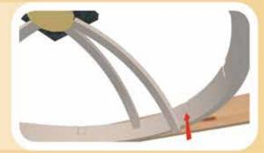
10. Nail or screw the dome rafters to the dome tie and to the dome ring using 2 nails or screws for each end.
