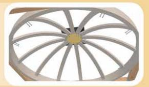
If you'll be hanging a heavy chandelier from the apex of 11. your dome, add a beam over the center of the dome tie and then nail or screw the dome tie into the beam.
