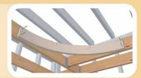
Nail or screw the square cut end of 2 dome rafters to the opposite ends of your dome tie using 2 nails or screws per dome rafter.
