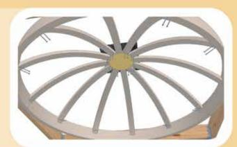
If you'll be hanging a heavy chandelier from the apex of your dome, add a beam over the center of the dome tie and then nail or screw the dome tie into the beam.
