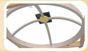
Install the remaining dome rafters by first butting the square cut ends to the dome tie and then sliding the miter cut ends up the dome ring unit they "snap" into the rafter holsters.
