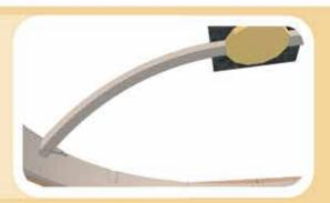
Nail or screw 2 dome rafters perpendicular to the first 2 dome rafters to both the dome tie and dome ring using 2 nails or screws per dome rafter for each end. This will keep the dome tie rigid when installing the remaining dome rafters.
