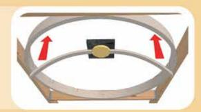
6. Nail or screw the miter ends of the 2 dome rafters into the dome ring using 2 nails or screws per dome rafter.
