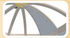
If necessary, trim off the excess drywall with a utility knife that overlaps the center line on both dome rafters.
