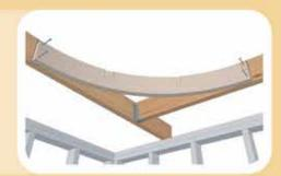
Nail or screw the square cut end of 2 dome rafters to the opposite ends of your dome tie using 2 nails or screws per dome rafter.
