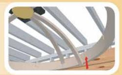
Nail or screw the dome rafters to the dome tie and to the dome ring using 2 nails or screws for each end.
