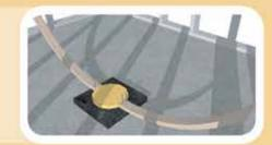
Slide the mitered ends of the 2 dome rafters into the rafter holsters.
